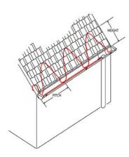
Use the following table to calculate the total number of metres required for a G-TRACE roof installation.
