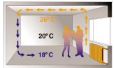
Room heating using traditional methods
