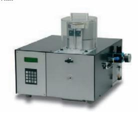
The CA 4/8 Indent is an electro-pneumatic-driven automatic stripper and crimper for processing loose-packed, . turned male and female contacts. The contacts are fed automatically via an oscillating conveyor set-up.
