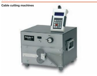
The CutFix 8 is a microprocessor-controlled tool for the automatic cutting to length of solid and flexible single conductors with a max. outer diameter of 8 mm.
