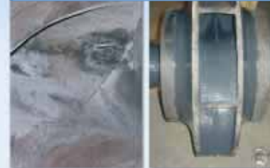
Impeller and casing before repair. Serious wear and cavitations on the impeller
