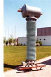
245 kV Current Transformer manufactured in 1975
