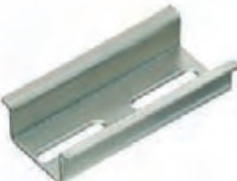
TS 35/15 mm according to EN 50022 (s = 1.5 mm)
