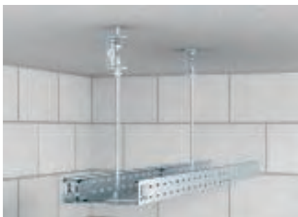
Direct centre suspension with threaded rod, type 2078/M10. This mounting variant is possible for RKS cable trays of width 50 to 200 mm.
