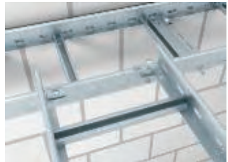
Creation of a horizontal tee exit of two cable ladders at different heights. The support angle, type LAW, is required to fix two cable ladders.
